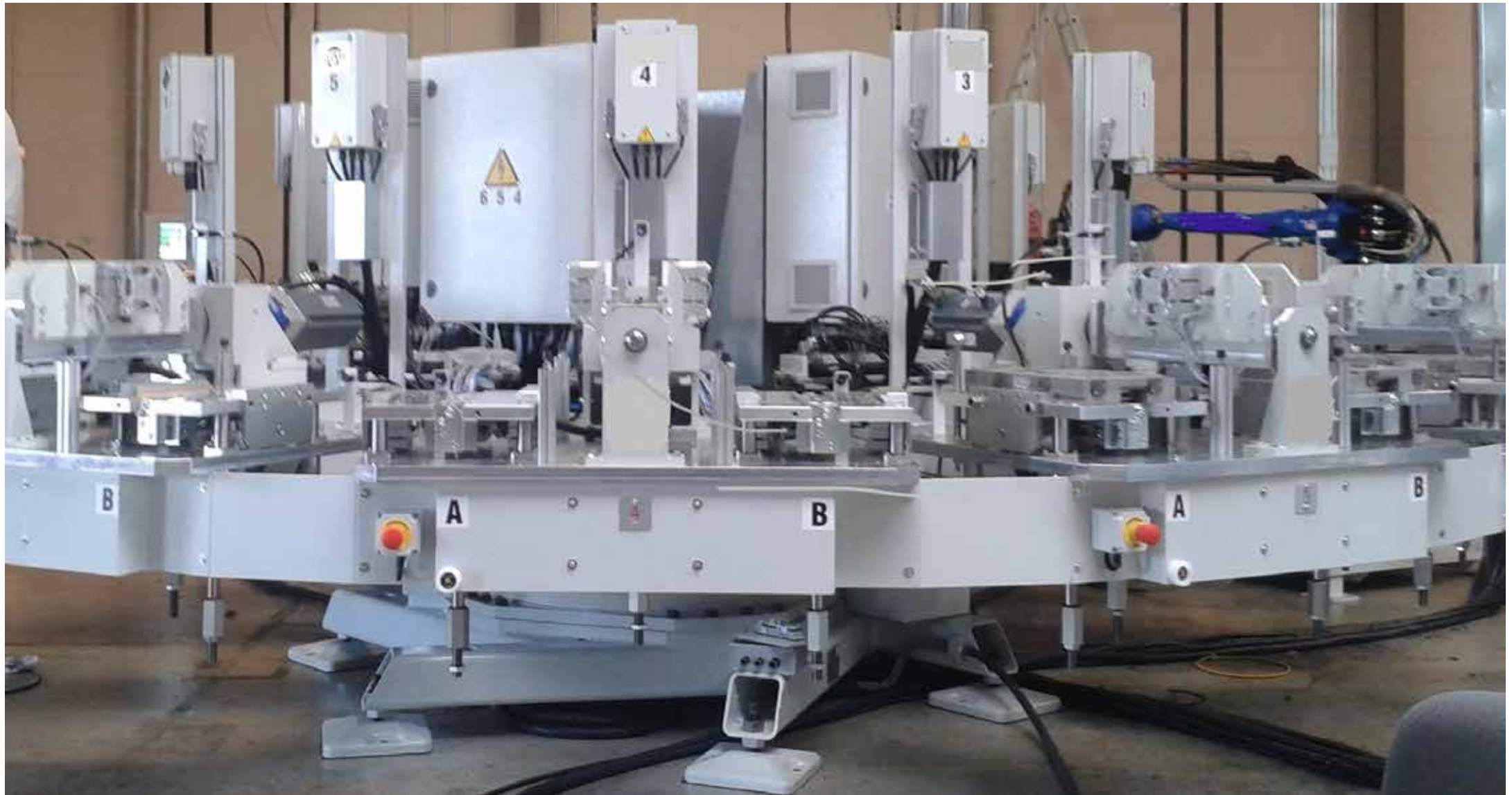
Use of variable pitch rotary table for polyurethane molding machine.
